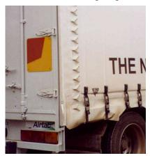
Airtabs are the only way to effectively deal with drag created in the gap between prime mover and trailer. Airtabs have no impact on your turning circle or fifth wheel location.
